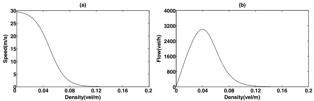
**Fig. 1** The speed-density and flow-density relationships in the classical fundamental diagram theory
