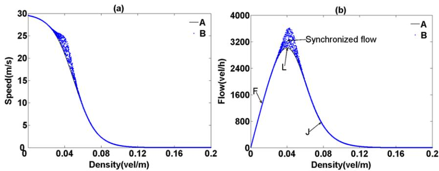
**Fig. 4** The speed-density and flow-density relationships of equilibrium flow, where the curves “A” are the equilibrium speed-density and flow-density curves of the classical funda-
