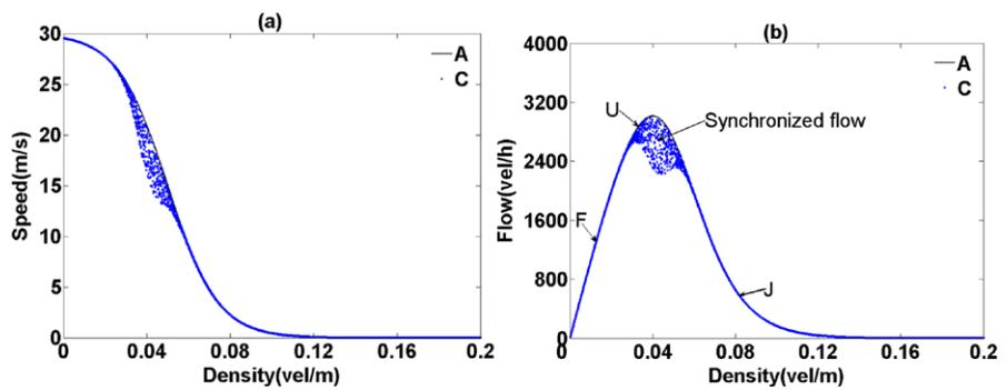
**Fig. 6** The speed-density and flow-density relationships of equilibrium flow, where the widely scattered data “D” are the widely scattered speed-density and flow-density data when the traffic system simultaneously has the conservative and aggressive drivers
