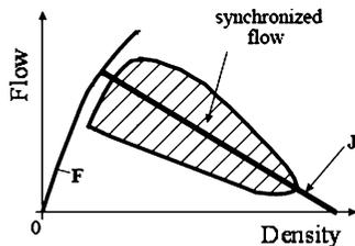
**Fig. 2** The flow-density relationship in the three phase traffic flow theory [2]
