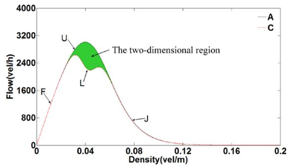
**Fig. 9** The boundary line of the flow-density relationship, where the curves A and C are the same as those of Fig. 5
