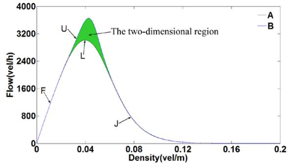
**Fig. 8** The boundary line of the flow-density relationship, where the curves A and B are the same as those of Fig. 4
